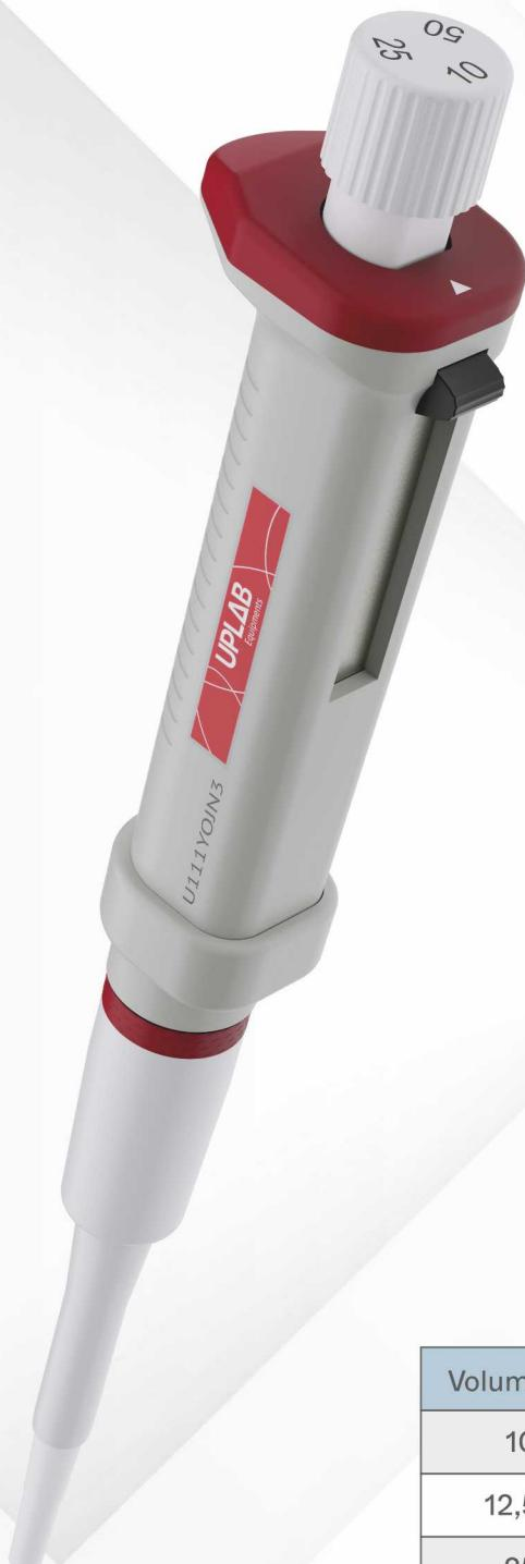
The UPLAB repetitive micropipette device is designed for precise transfer of liquids in a laboratory environment. The device provides dispensing volumes that can be adjusted to 10-12.5, 25, and 50  $\mu\text{l}$ , ensuring accurate and consistent transfer of samples.
